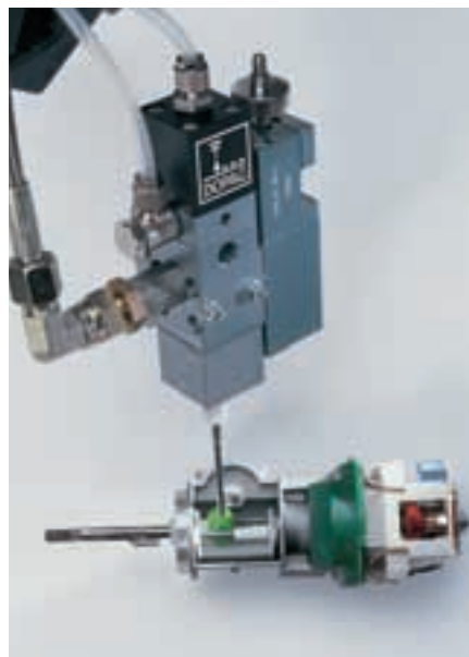
Lifetime lubrication of gears
