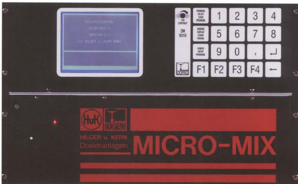
▲ MICRO-MIX S metering computer
